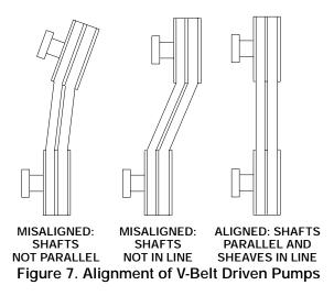
Tighten the belts in accordance with the belt manufacturer's instructions. If the belts are too loose, they will slip; if the belts are too tight, there will be excessive power loss and possible bearing failure.
